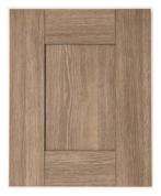
Our shaker doors are constructed of five separate RAUVISIO panels assembled with REHAU LaserEdge on all four sides. The 3" wide frame (stiles and rails) consists of %" thick material and the center panel consists of %6" thick material. Maximum warrantied size is 30 in W x 65 in H (762 mm W x 1651 mm H), any height over 48 in (1219.2 mm) requires a center rail.
