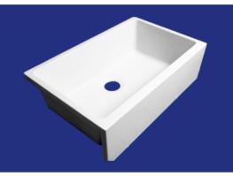
The FS3019-S can be top mounted, or under mounted on any type of countertop surface. The bottom of the sink allows it to be easily supported for easy installation. The front apron can be trimmed, allowing it to be custom sized to fit any standard drawer front.
