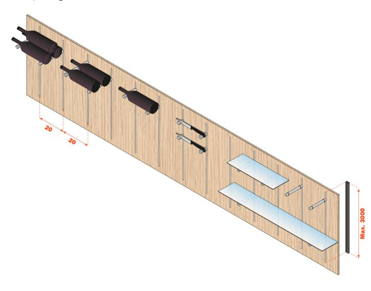
When machining the wood panel, leave 100 mm from the top and from the bottom of the panel.
