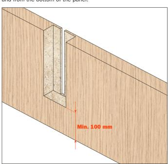
Dimensions for machining the panel.
