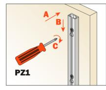
Drilling the wood panel to fix the surface-mounted profile. Use the screws supplied with wall plugs.
